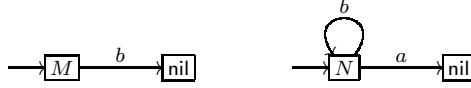
Fig. 4. From left to right: LTS(M) , M = b.nil , and LTS(N) , N = rec_x(b.x + a.nil) .
